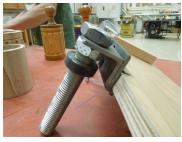
The three phots below show the index wheel pointer and mount. The pointer is bolted into the base, which sits on the lathe bed rails and held with magnets. The pointer height has a slight adjustment range depending on the index division set used. The wheel is not shown, but mounts on the spindle
