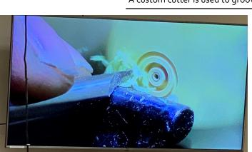
Above, the blank is mounted on the chuck insert using the two pins to register the blank position. The grooves are cut to the depth of the intersection plane between the work performed from the front and rear faces of the blank.
