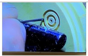
Here Hans measures the depth of the grooves cut first on the front face. After cutting the front face the part is flipped and grooved on rear face
