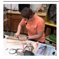
Once the body sections are turned and hollowed, the off center contours are added. Here Rebecca shows the method she uses to power carve the contours on the top section.
