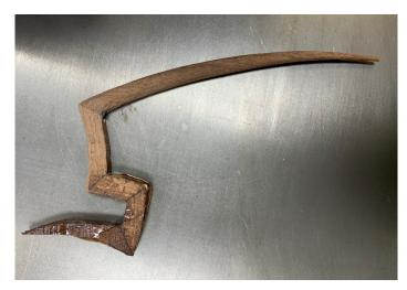
Leg that has been assembled from sections to enable the complex shape to be achieved
