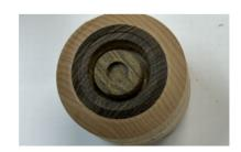
4. Use a blank for the lid with a diameter slightly larger than the recess made in the box. Make a jamb fit with the box.
