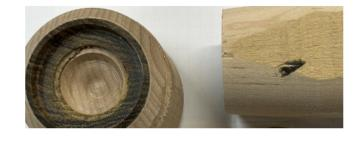
5. Use the box in the chuck to hold the lid. Drill a 1/4 inch hole 1/4 inch deep. Turn the top of the lid and bottom of the finial.
