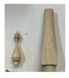
8. Make a Jamb chuck to reverse the box. Finish the bottom of the box, leave a tenon to receive the foot blank. Turn and finish the foot.
